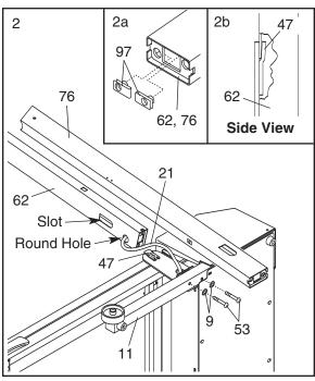
3. With the help of a second person, tip the treadmill so the Base Pads (40) (see drawing 1) are laying flat on the floor. Raise the Uprights (62, 76) to the vertical position.
